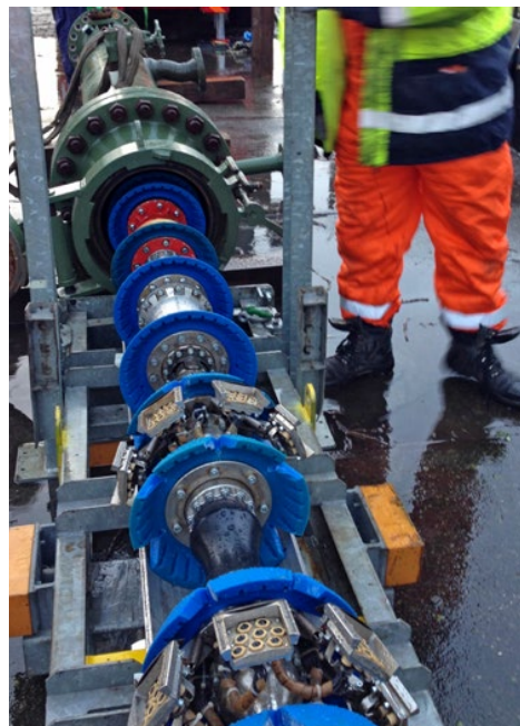
The intelligent PIG (Pipeline Inspection Gear), a tool to internally inspect the condition of the pipeline.
