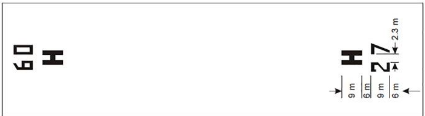
Figure F-2. FATO designation marking and heliport identification marking for a runway-type FATO
