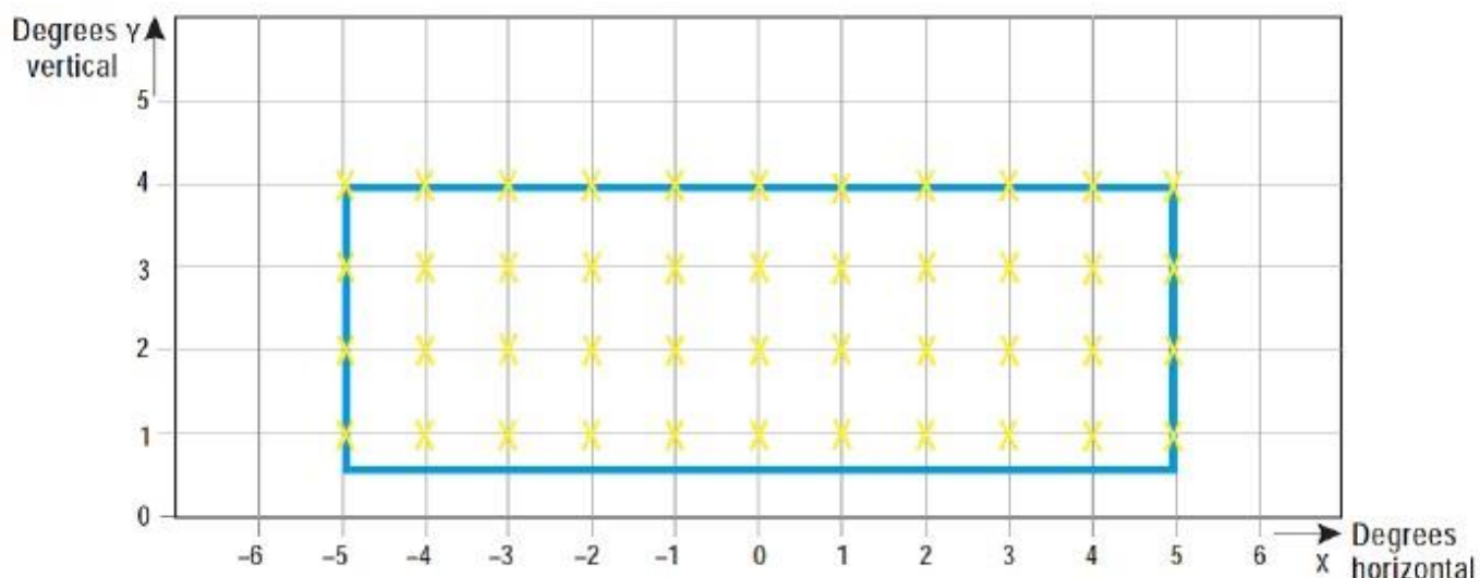
Figure U-25. Grid points to be used for calculation of average intensity of taxiway centre line and stop bar lights
